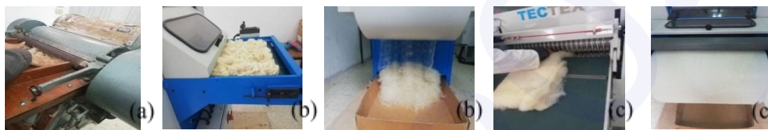
Figure 1: The steps for the synthesis of the non-woven abrasive: (a) opening of the fibers by Shirley machine (b) formation of the sail by the card (c) mechanical consolidation using a needling machine
