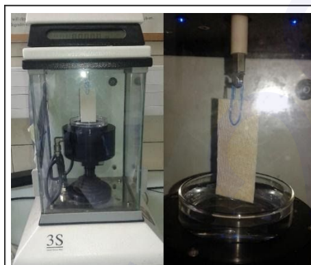
Figure 2: Used GBX-3S Tensiometer and a suspended sample with its bottom end dipped in distilled water.
